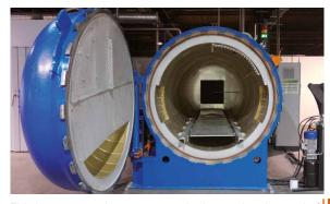
This investment aims to answer the increasing demand of our clients in the development and the manufacturing of composite structural parts. This autoclave completes our current means to apply different manufacturing process (RTM injection machine, Oven, Press). This new equipment allows us to provide an efficient polymerization process integrating temperature, pressure and vaccum.
