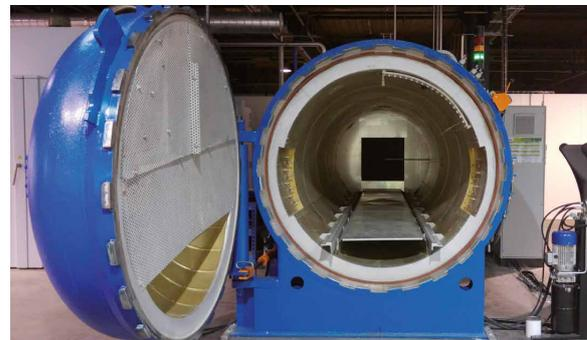
This investment aims to answer the increasing demand of our clients in the development and the manufacturing of composite structural parts. This autoclave completes our current means to apply different manufacturing process (RTM injection machine, Oven, Press). This new equipment allows us to provide an efficient polymerization process integrating temperature, pressure and vacuum.
